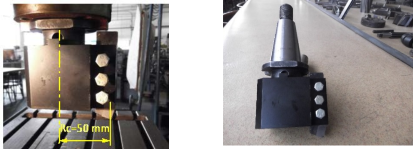
Fig. 7 – Fly cutter utilized for face milling.
